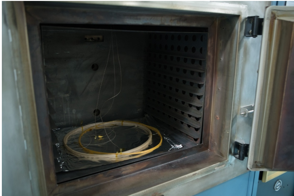
Figure 5: Testing scheme for elevated temperature cycling measurements showing placement of fiber optic coils in the furnace.
